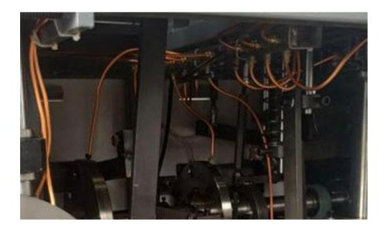
The machine automatically refuels the positions that need to be refueled through the copper pipe, saving
