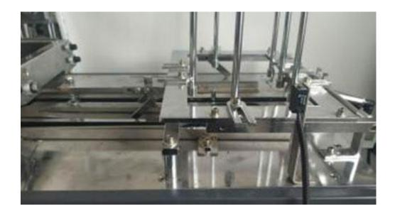
Three times of paper feeding, multiple mediation, to avoid unevenness on both sides of the paper cup.
