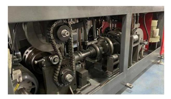
Disposable paper cup machine It has over-cup detection, cup-tube forming detection, and automatic shutdown alarm for faults. The process flow of the equipment is as follows: suction sheet→cup tube bonding→upper cup tube→upper cup bottom→preheating 1→preheating 2→bottom folding→knurling→hemming→lower cup→rewinding
