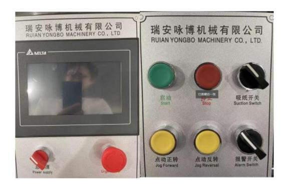
This **Disposable Paper Cup Machine** Control panel with good quality switches, temperature controller and speed converter. All the operation of machine can be finished easily by this panel.
