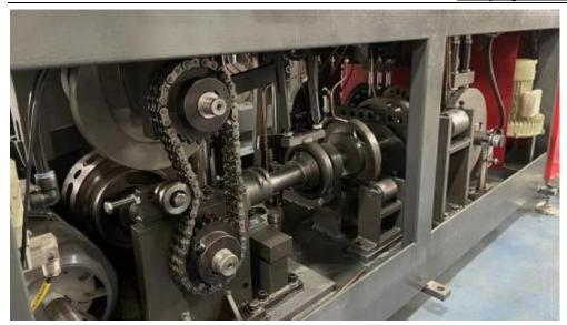
1. The whole **Disposable Paper Cup Machine** adopts automatic oil lubrication system(oil circulation system is including oil motor, filter, copper pipe ) which makes all gear moving parts working at high speed much more smoothly and greatly Improve the service life of spare parts.
